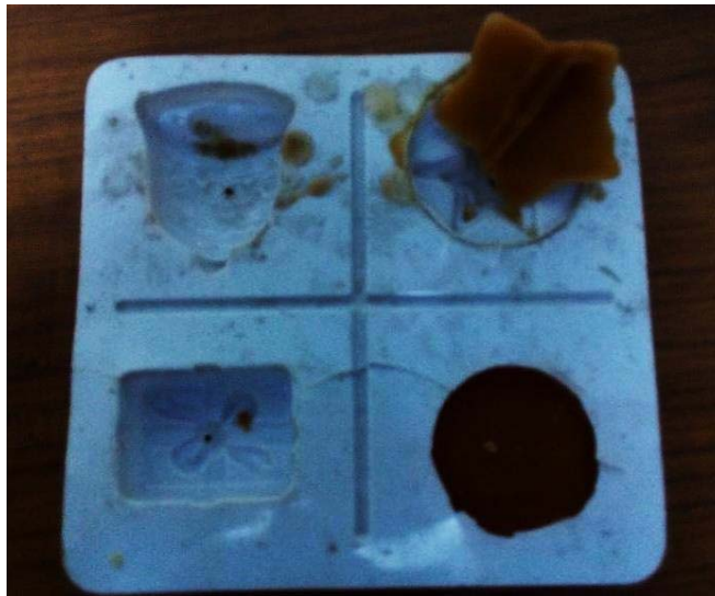
Figure 6.1: Various wax shapes to be used for investment casting
