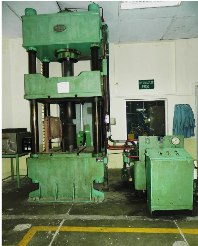
Figure 2.2: A typical Forging press (open die forging)
