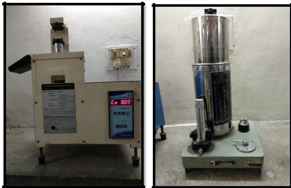
Figure 3.1 (left) Universal strength tester used for measuring compressive strength and shear strength; (right) Permeability testing equipment
